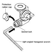
2. After loosening the bolt, hit the top of the wrench lightly. Hitting the wrench lightly will unlock the bolt and make it free to change installtion angle. Then adjust the bracket to make it vertical to road surface. To push lock nut at the oposite end will lock the bolt again. And hitting the bolt at the oposite end with the wrench will unlock the bolt.
